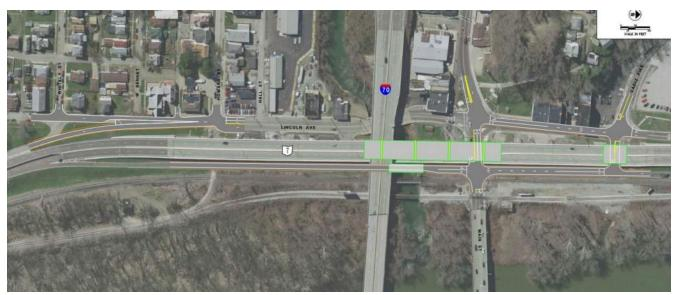
Figure 2 - Conceptual Schematic of the Tight Diamond Interchange Configuration
