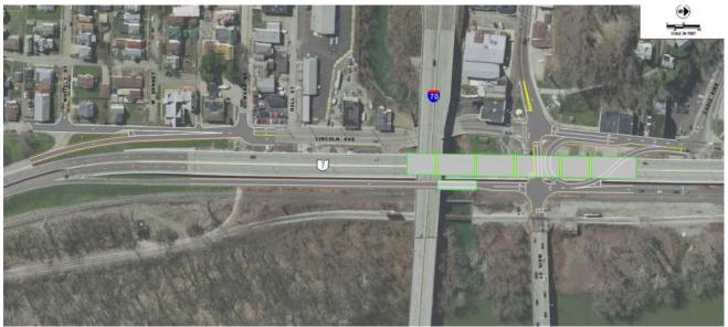
Figure 3 - Conceptual Schematic of the Tight Diamond with U-turn Interchange Configuration
