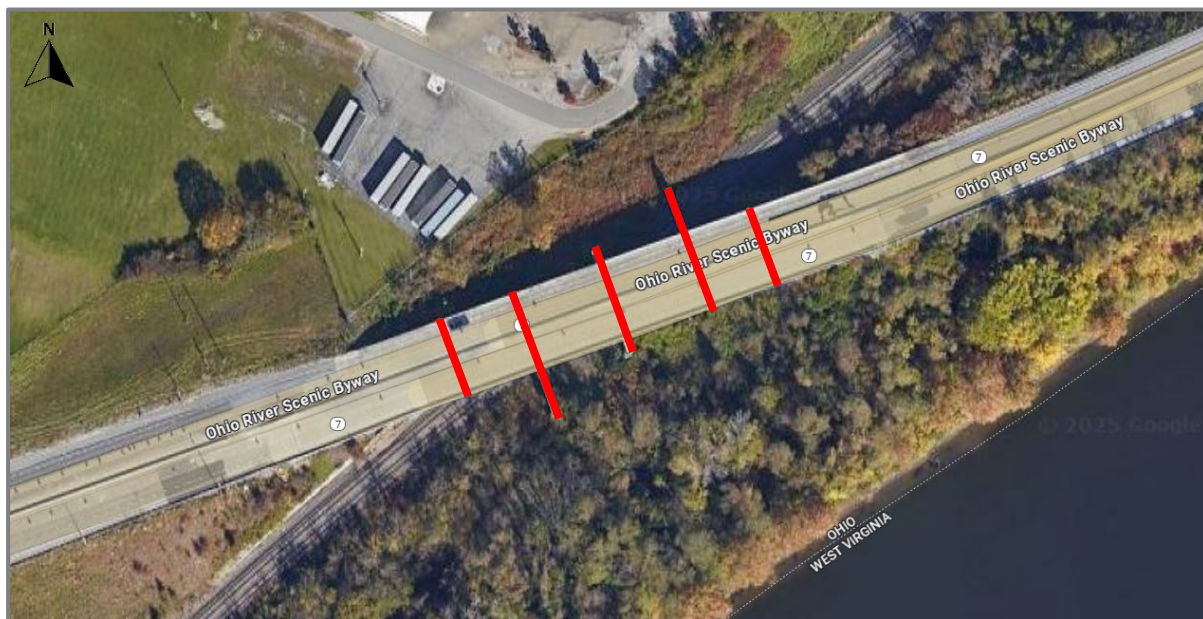
Figure 3 – NSTM Member Identification Plan (location of NSTM members highlighted in red).
