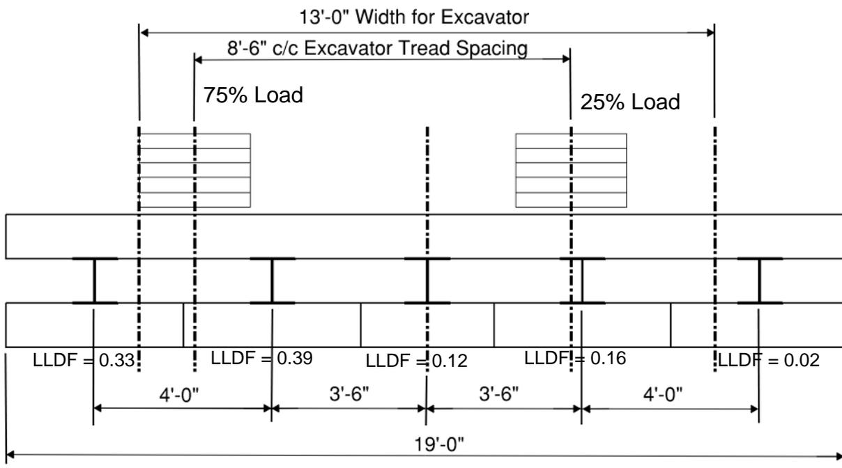
Case 2: Excavator Tread Centered on Beam. Max LLDF's Shown
