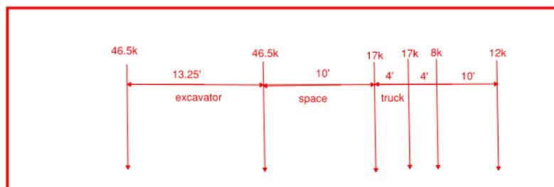
Assume Excavator is confined to the center of the crane mats, for design purposes assume it moves within a 13' width at the center of the crane mat. What is worst case LLDF? Still consider 75% of the load on a single tread. Tie rods installed before steel beams and crane mat placed. No different than a noncomposite slab beam/box beam bridge from a LLDF perspective.
