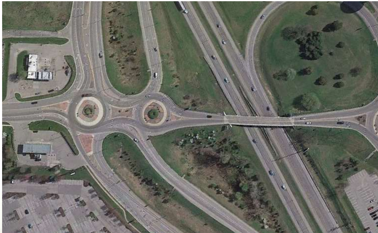
Figure 9 – Plan View of Double Roundabout at US 23 & Lee Road Interchange, Livingston, MI
