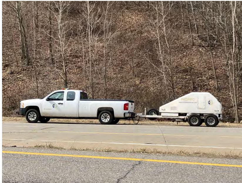
Photograph 2. FWD system used during data collection
