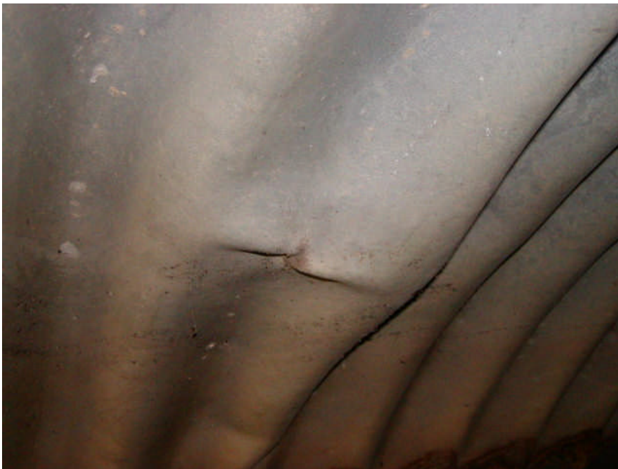
Photo 4. Indention in pipe number 3.
