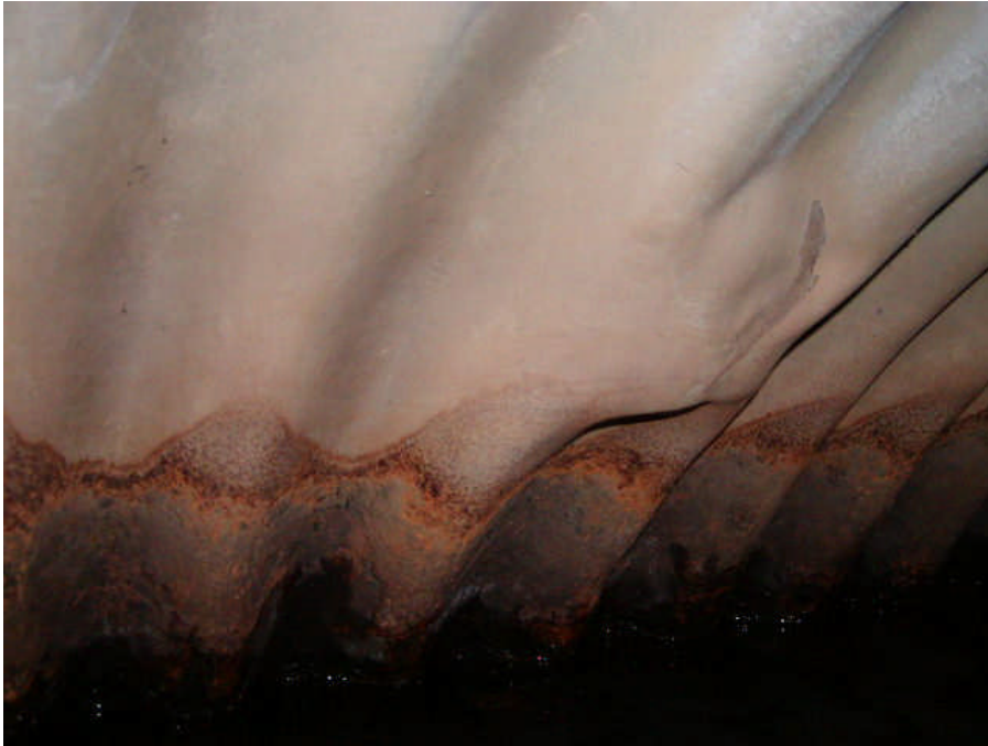
Photo 3. Indention in pipe number 1.
