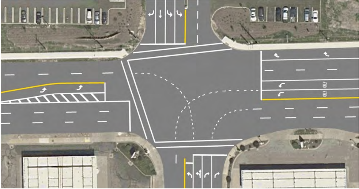
Figure 2. Plan view of Howe Rd. and State Route 82, showing existing lane use.
