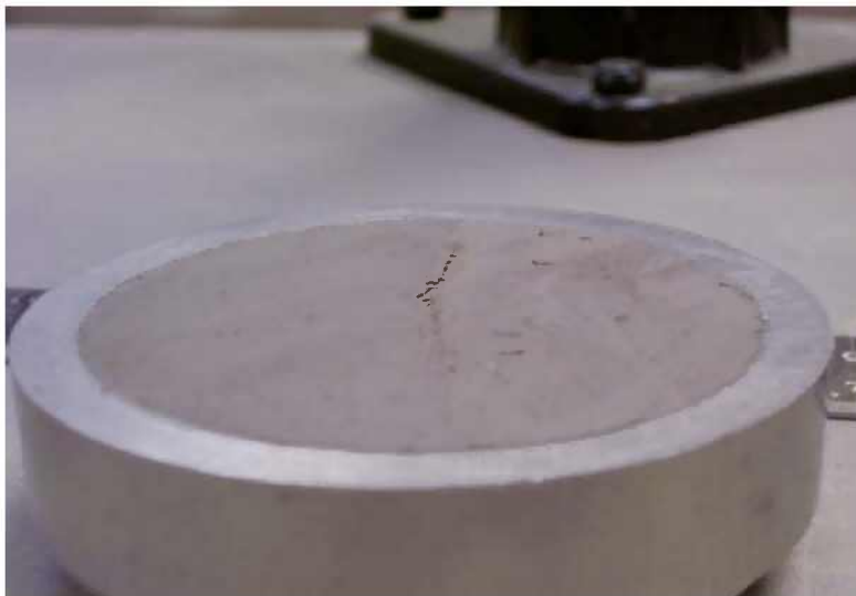
Sample in trimming ring showing an in-situ shear plane in the material as received. Residual Shear test (RS-2), angled view.
