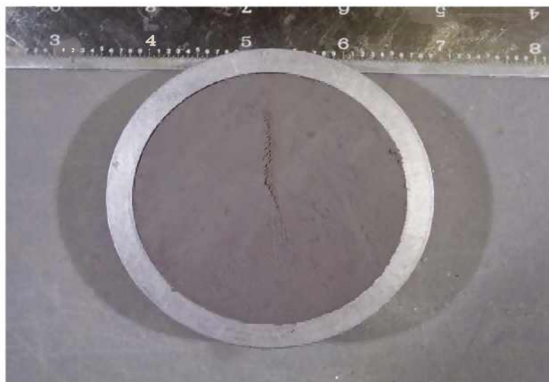
Same sample, in trimming ring showing an in-situ shear plane in the material as received. Residual Shear test (RS-2), top view.
