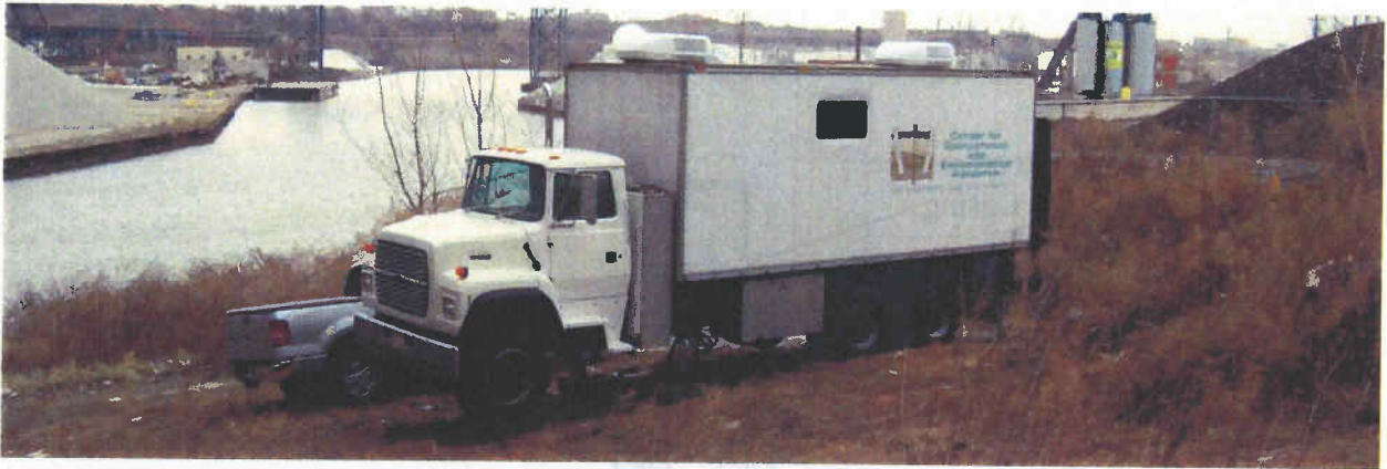
a) Cone Penetration Testing at C-05-03.
