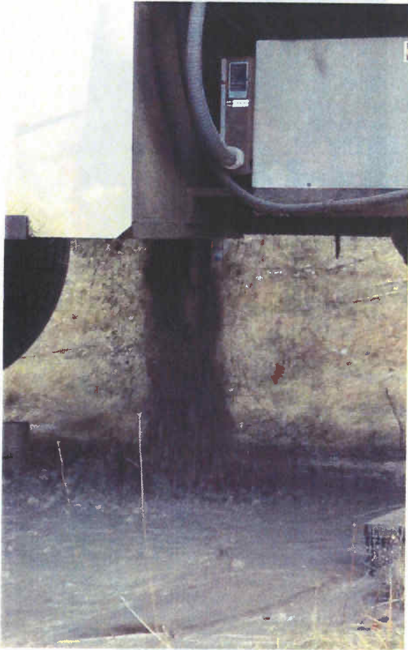
a) Water/gas erupting beneath the CPT rig at C-05-02.
