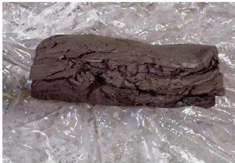
Same sample, broken to show the cross section through the middle of specimen. Shows horizontal layers, some with an almost blocky structure at a very small scale.
