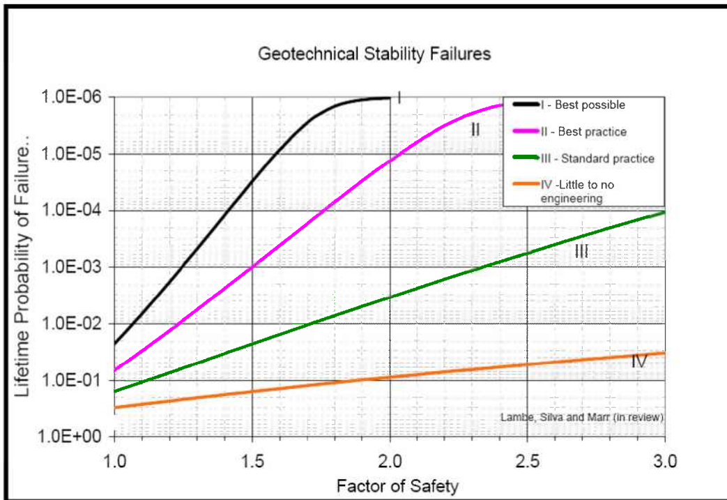
Figure 7B.11: Current version of Factor of Safety/Probability of Failure Curves (Lambe, Marr, Silva - in review)
