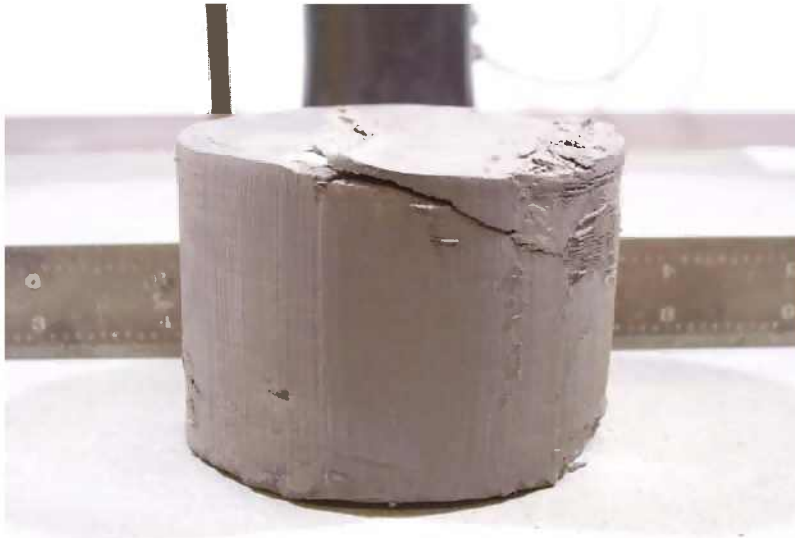
Extruded sample showing in-situ shear plane. Side view. Direct Simple Shear test, DSS-2 was trimmed from this piece.
