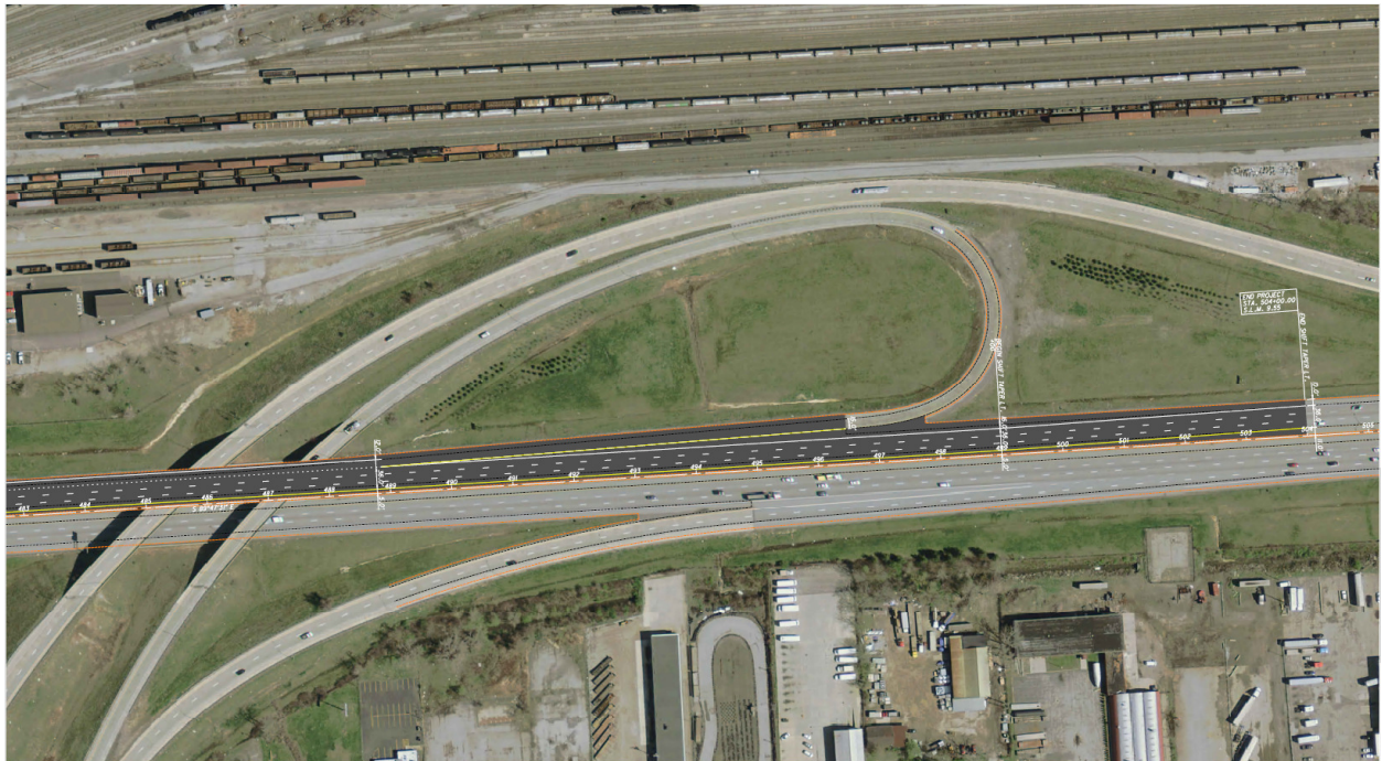
Figure 5. I-71 NB exit to I-480 WB becomes an auxiliary lane with a weave section rather than an acceleration lane with a merge.
