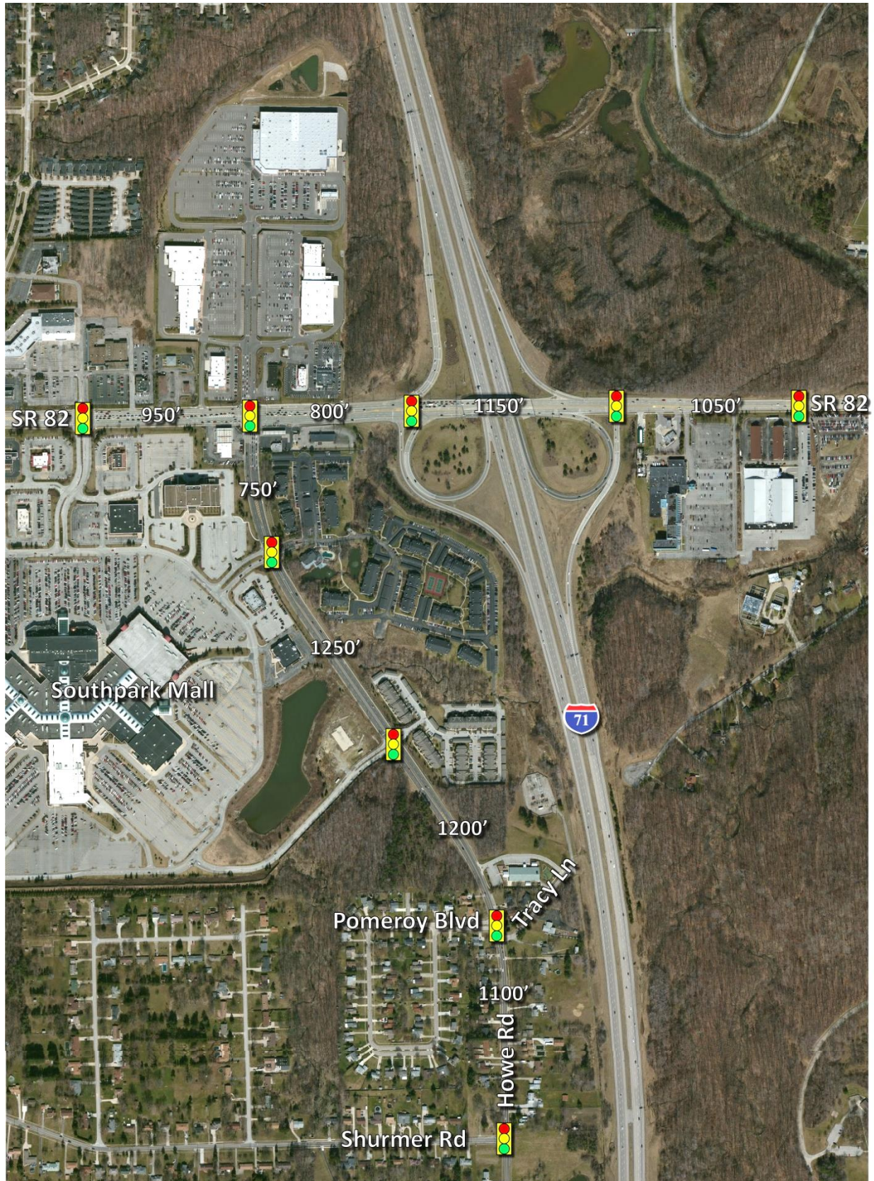
Figure 4 - I-71/SR 82 Interchange with Signal Spacing
