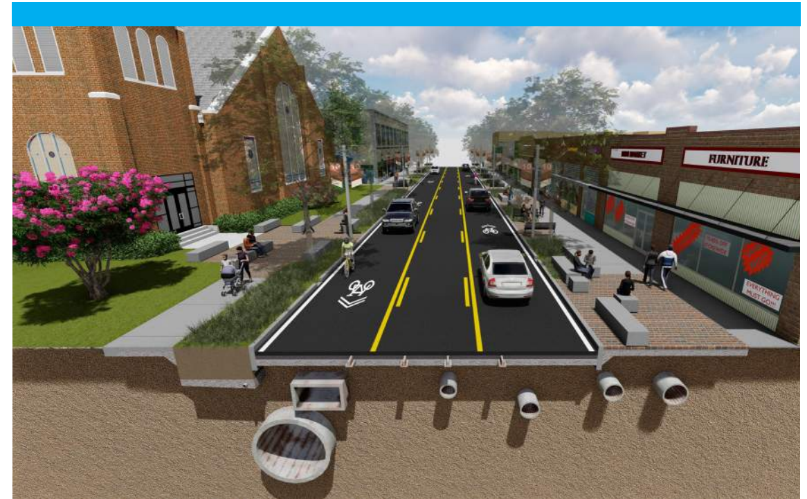
60' Right of Way with Expanded Sidewalk
