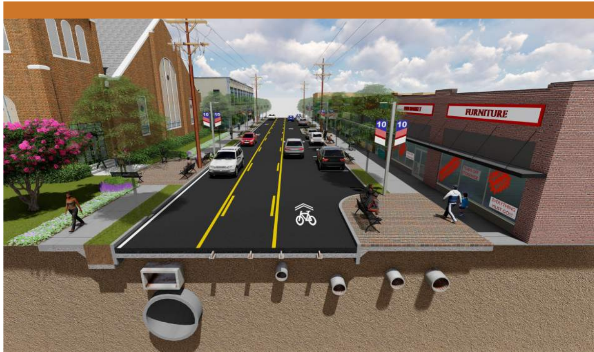
60' Right of Way with On-Street Parking
