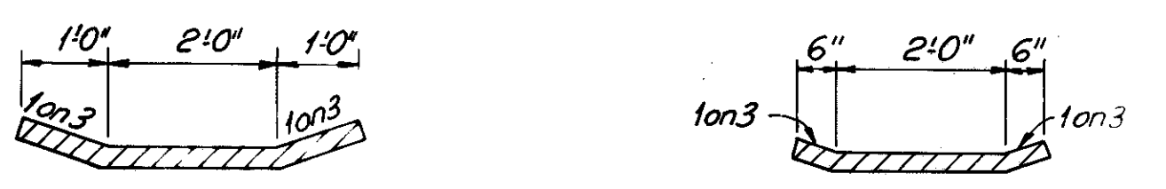
SECTION OF SODDED DITCH D-17 D-17 54+75 to 57+00 N.B. Jennings Rt. SECTION OF SODDED DITCH D-18 D-18 58+00 to 58+50 N.B. Jennings Rt.
