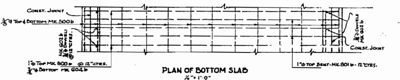
BAR LIST - TYPICAL SECTION N#2 - 12'-0" x 5'-0" REINFC. CONC. CULVERT
