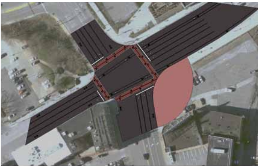
PROPOSED GRADE LEVEL IMPROVEMENTS at the corner of W. 25th & Detroit Ave. showing an all purpose trail designation at all four corners of the intersection
