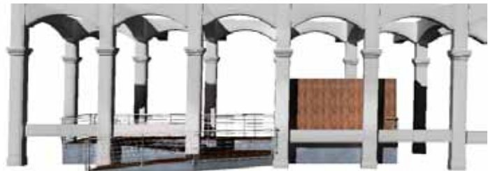
INSTALLING PLATFORMS where lower crossbeams are not present avoids additional structural configuration.
