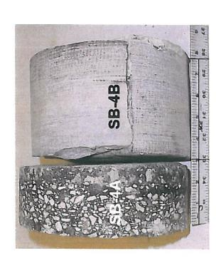
3" Asphalt Concrete; 4.5" CONCRETE
