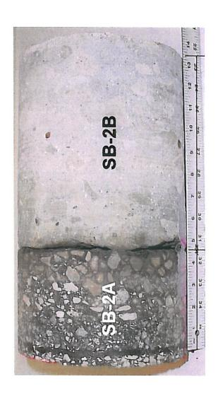
4.5" Asphalt Concrete; 9" CONCRETE
