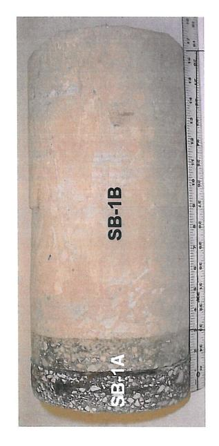
3" Asphalt Concrete; 13.5" CONCRETE
