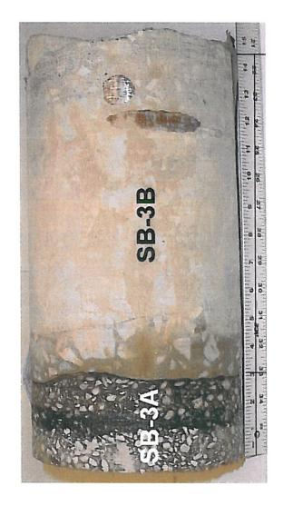
3" Asphalt Concrete; 11.5" CONCRETE
