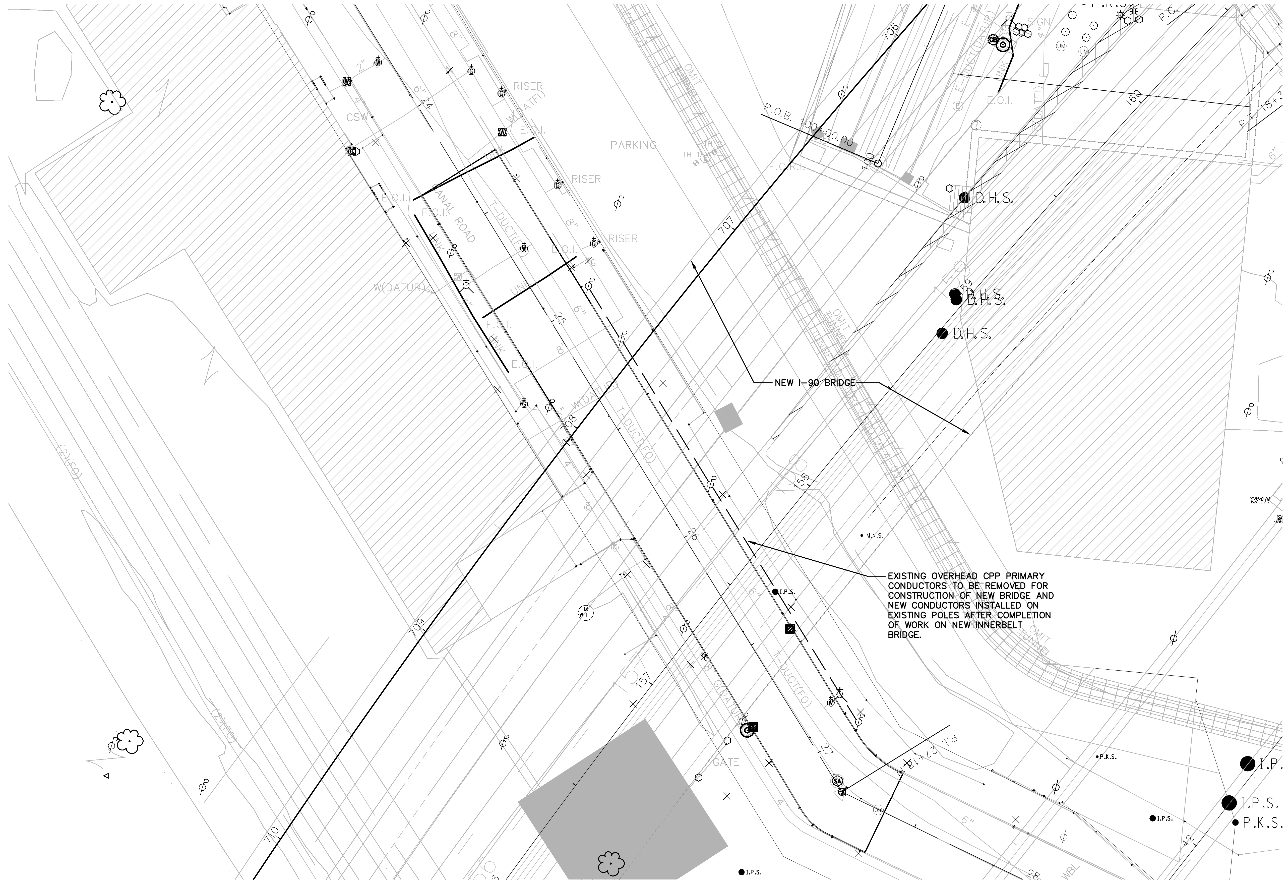
CANAL ROAD POLE RELOCATION SCALE: 1"=20'
