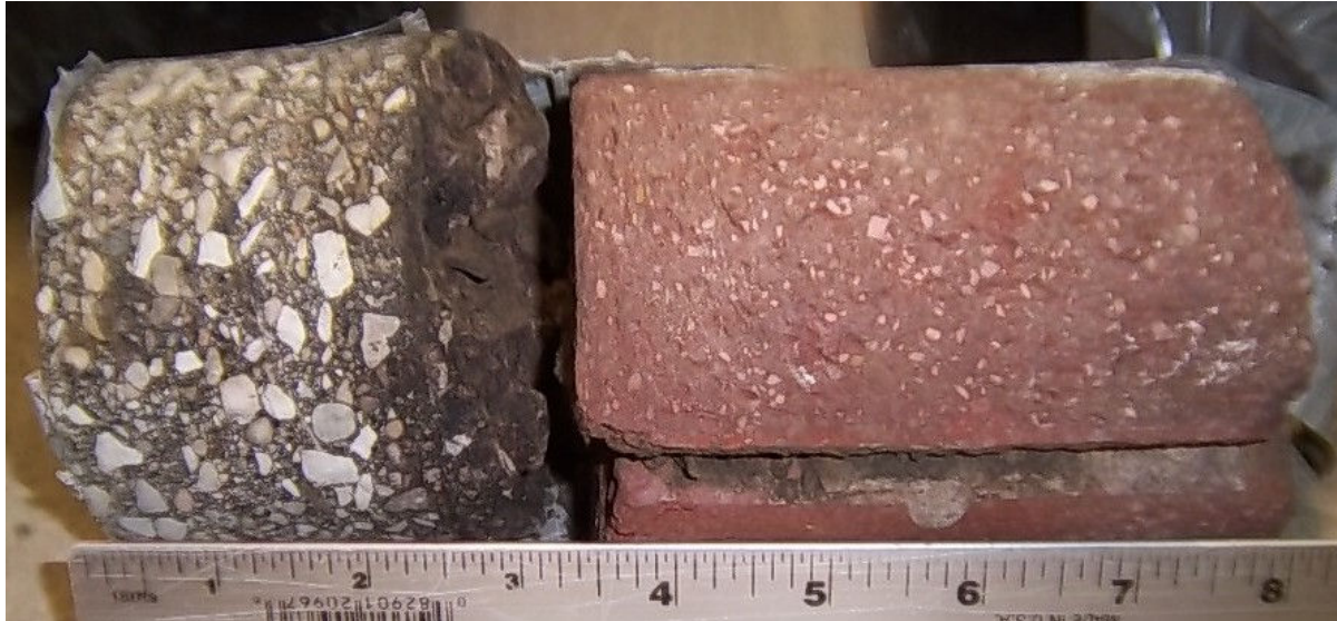
Core #32 Location: NE, Center on Literary Ave. 3 1/2" Asphalt / 4 1/2" Brick
