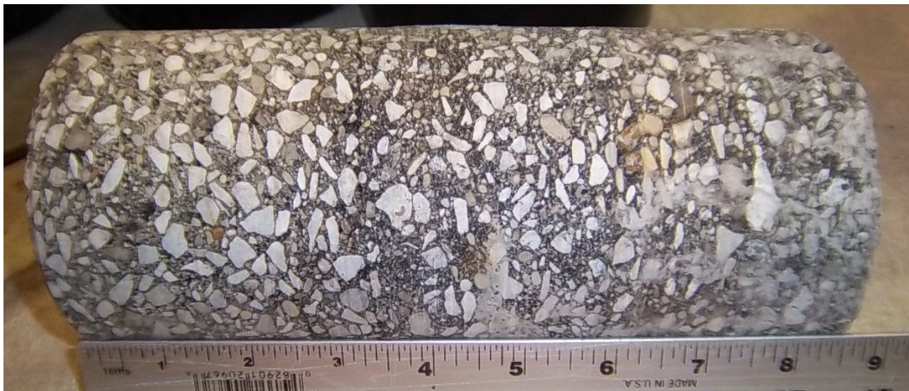
Core #41 Location: SE, Center on Professor Ave. 8 ½" Asphalt
