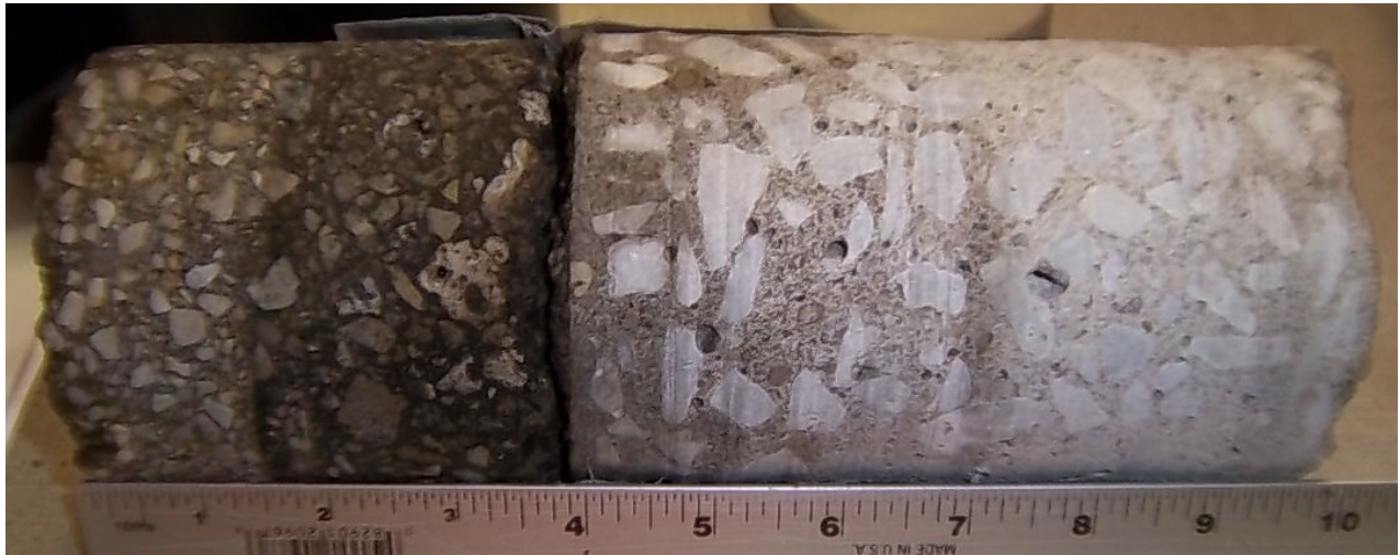
Core #26 Location: North Center of Intersection 3 7/8" Asphalt / 6" Concrete
