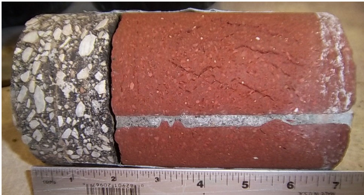
Core #39 Location: SW, South on Literary Ave. 2" Asphalt / 5" Brick
