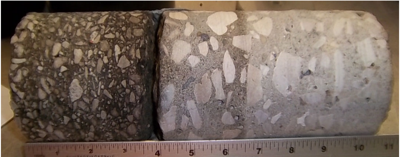
Core #28 Location: South Center of Intersection 3 ¾" Asphalt / 6 ¾" Concrete
