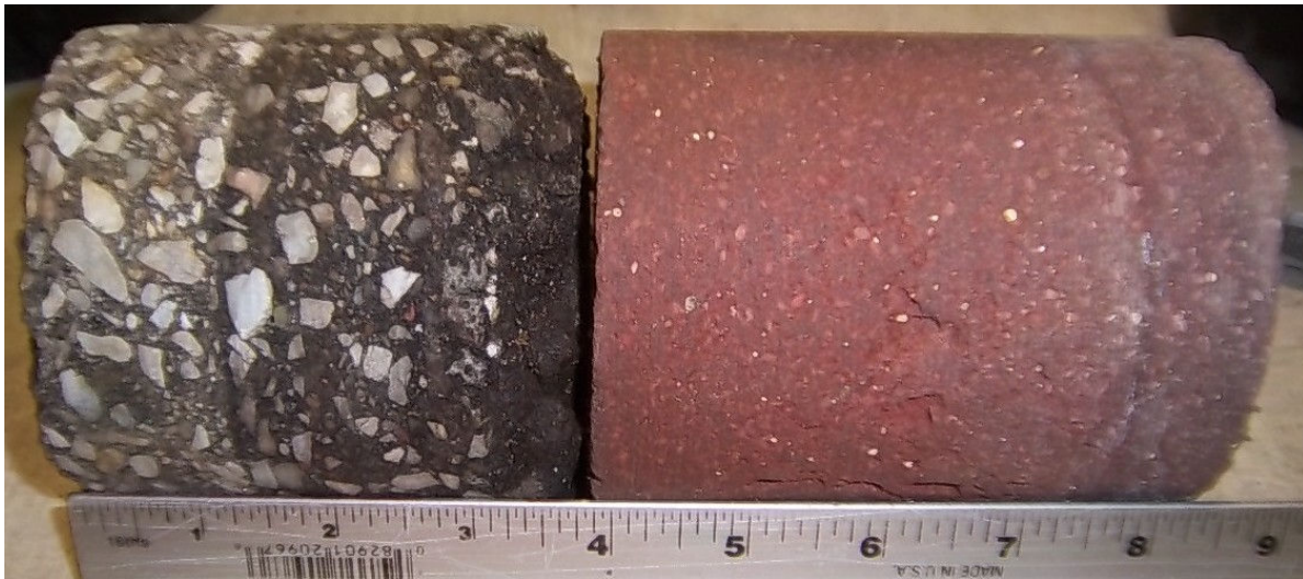
Core #33 Location: NE, East on Literary Ave. 3 7/8" Asphalt / 4 5/8" Brick
