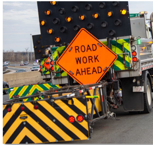
Figure 3: TMA with Connected Arrow Board
