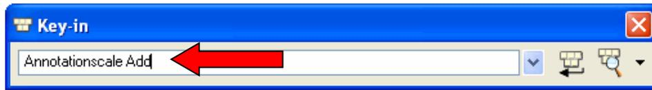
This command will apply the annotation scale to all the cells and text in the model. The cells and text will now take on the active model annotation scale value.
