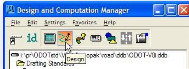
The **Design** mode is used to plot COGO elements into MicroStation, with the desired symbology, by use of the Draw Plan and Profile dialog box. It can also be used to set drafting standards used in conjunction with MicroStation's element placement commands, with the **Place Influence** option *toggle*d on, as shown below:
