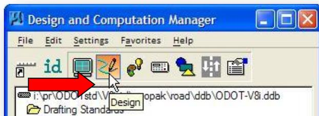
The **Design mode** is used to plot COGO elements into MicroStation with the desired symbology by use of the Draw Plan and Profile dialog box. It can also be used to set drafting standards to be used in conjunction with MicroStation's element placement commands, with the **Place Influence** option **toggle**d on, as shown below:
