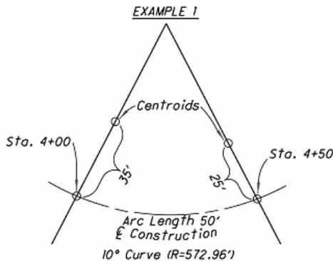
**EXAMPLE 1:** Find corrected arc length where centroids are located inside the curve.
