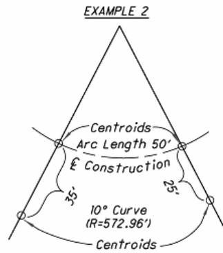
**EXAMPLE 2:** Find corrected arc length where centroids are located outside the curve.
