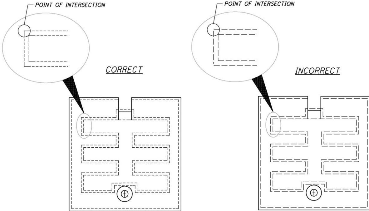
When needed for clarity, a gap should be shown at all locations where a visible edge becomes hidden by another surface as shown below.
