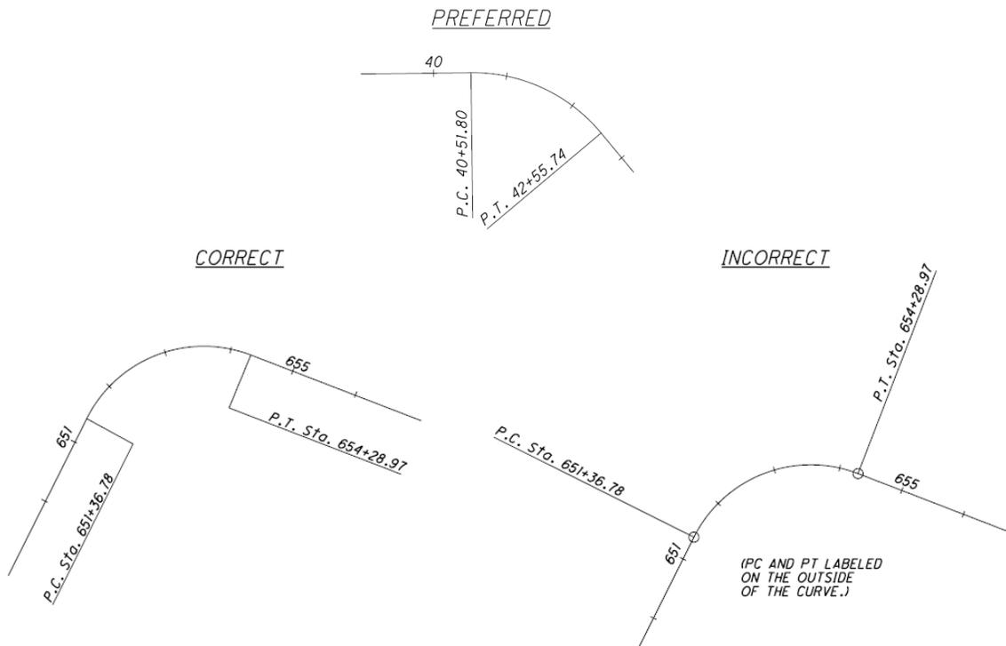
When space prohibits or when an alignment has a large number of horizontal curves, label each curve and tabulate the curve data. If it is necessary to tabulate curve data for a few curves along an alignment, then all curves should be tabulated to provide consistency.
