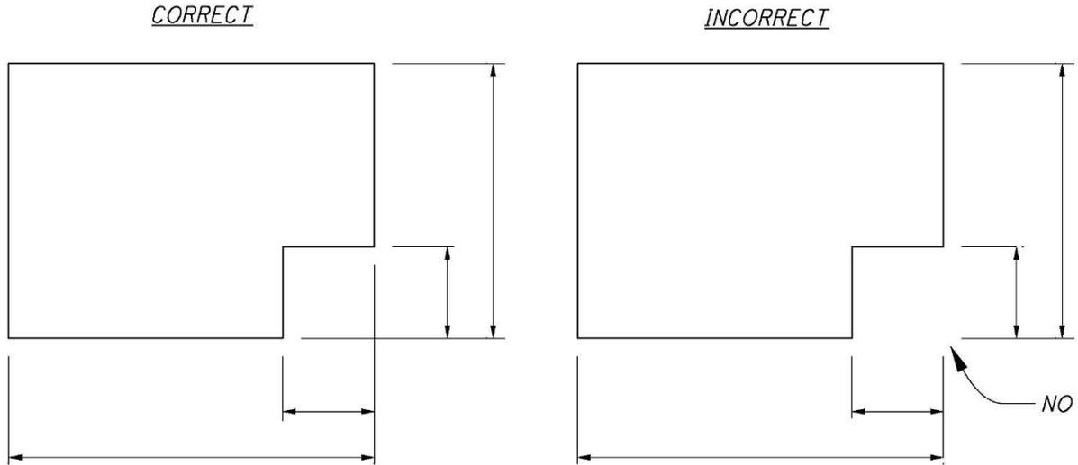
Extension lines should not be shortened. Also, a dimension line should never coincide with or form a continuation of any line of the drawing. If possible, dimensions should always be placed off the object.
