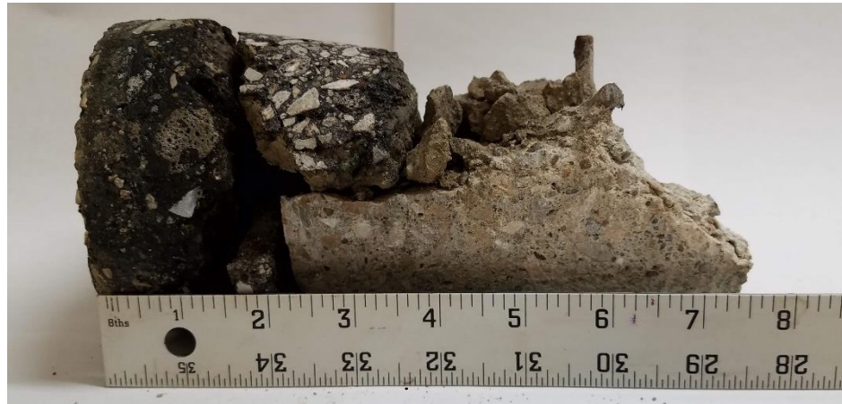
C-2 (5" Concrete, with 3 1/2" Asphalt Patch)
