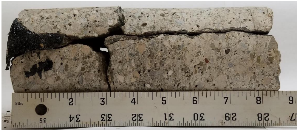
C-3 (8 1/2" Concrete, with 2 1/2" Asphalt Patch)
