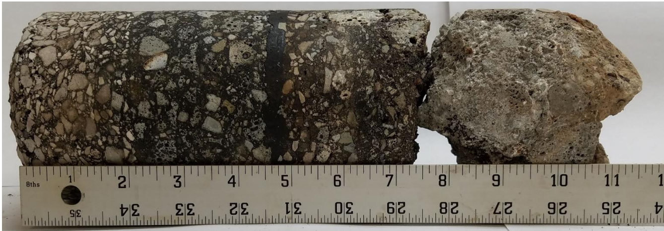
C-12 (7 1/2" Asphalt Concrete, 4" Concrete)
