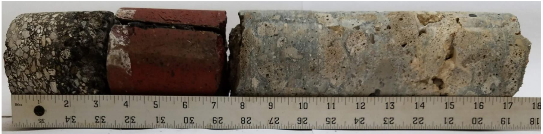
C-11 (3 1/4" Asphalt Concrete, 4 1/4" Red Brick, 10" Concrete)
