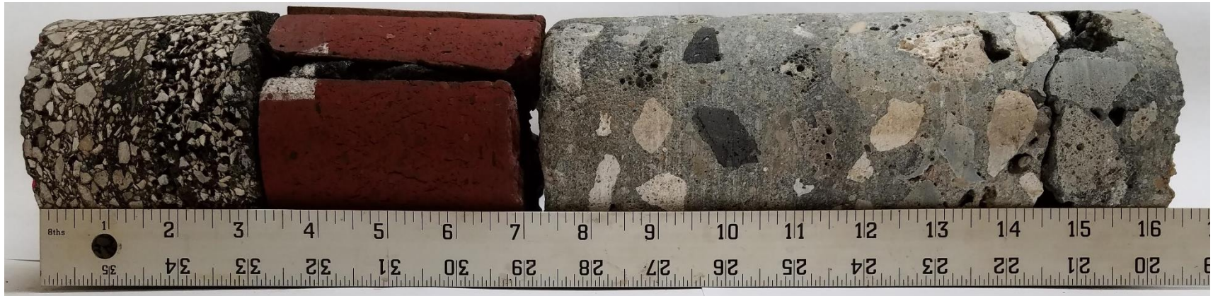
C-13 (3 1/4" Asphalt Concrete, 4" Red Brick, 9" Concrete)
