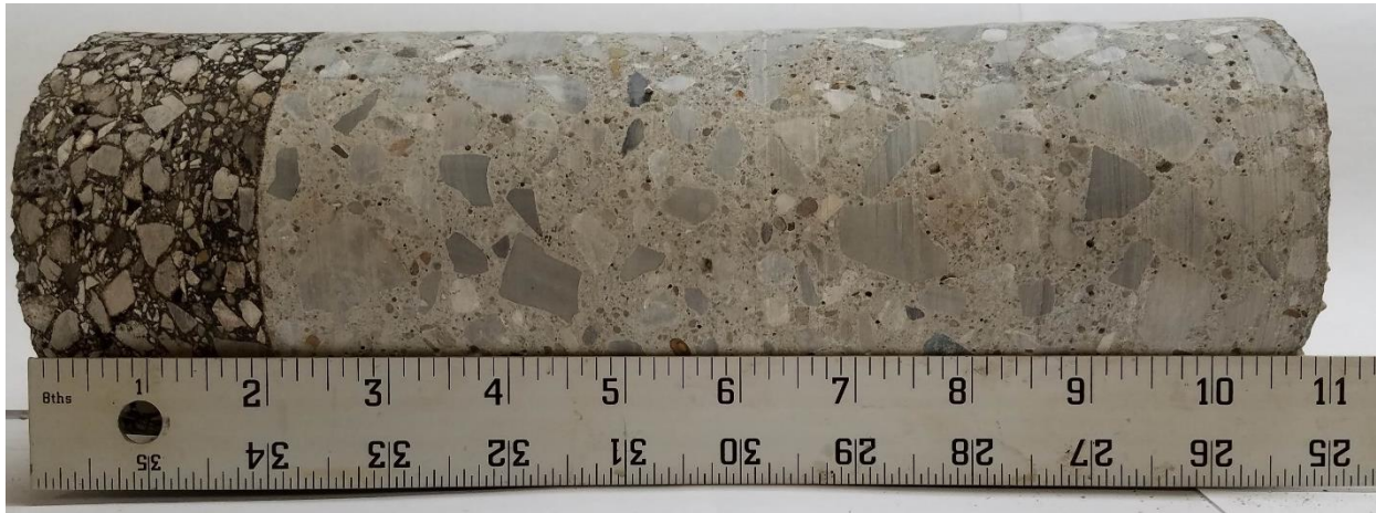
C-10 (2" Asphalt Concrete, 9" Concrete)
