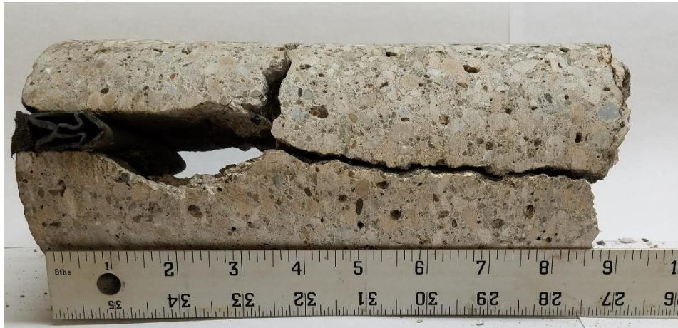
C-9 (9" Concrete, with Tar Paper Patch)
