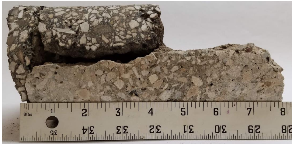
C-5 (7 3/4" Concrete, with 4" Asphalt Patch)
