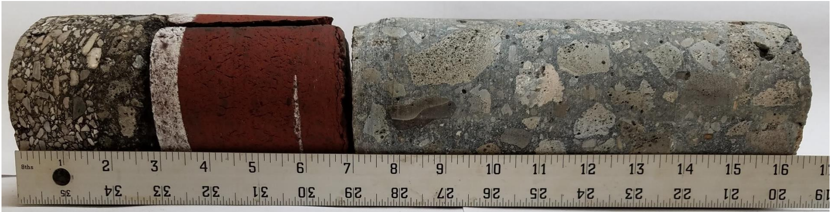
C-15 (3" Asphalt Concrete, 4" Red Brick, 9 1/2" Concrete)
