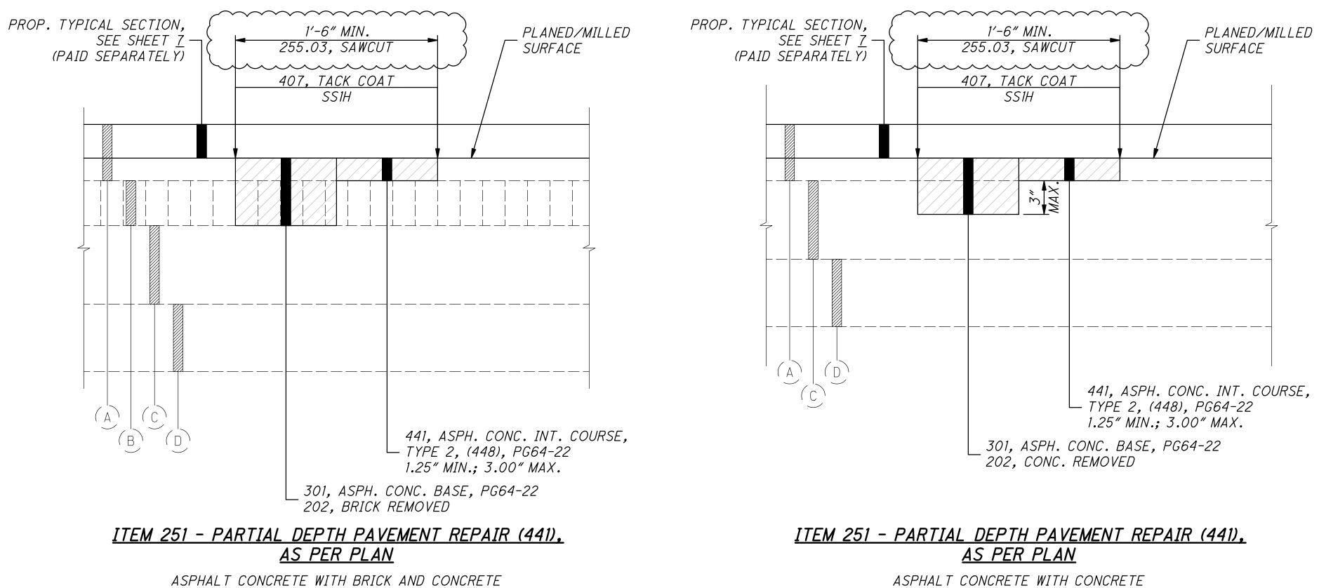
ASPHALT CONCRETE WITH CONCRETE
