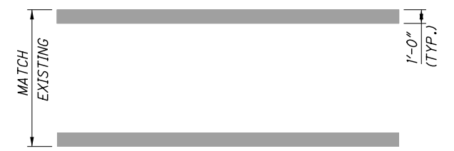
FINAL CROSSWALK MARKING DETAIL (LONGITUDINAL LINES ONLY)
