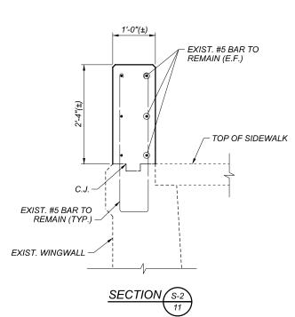
TYPICAL RAILING REPLACEMENT ON WINGWALL WINGWALL REINFORCEMENT NOT SHOWN FOR CLARITY
