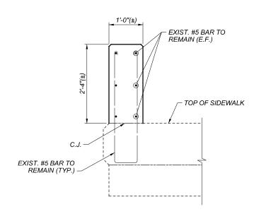
TYPICAL RAILING REPLACEMENT ON SUPERSTRUCTURE DECK REINFORCEMENT NOT SHOWN FOR CLARITY
