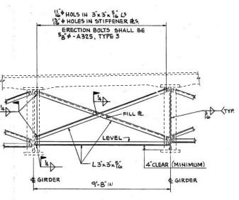
FRAMING DETAIL AT ABUTMENTS
