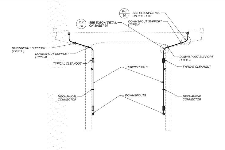
TYPICAL COLUMN DRAINAGE - ARCH SPANS
