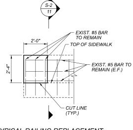
TYPICAL RAILING REPLACEMENT ON WINGWALL ELEVATION
