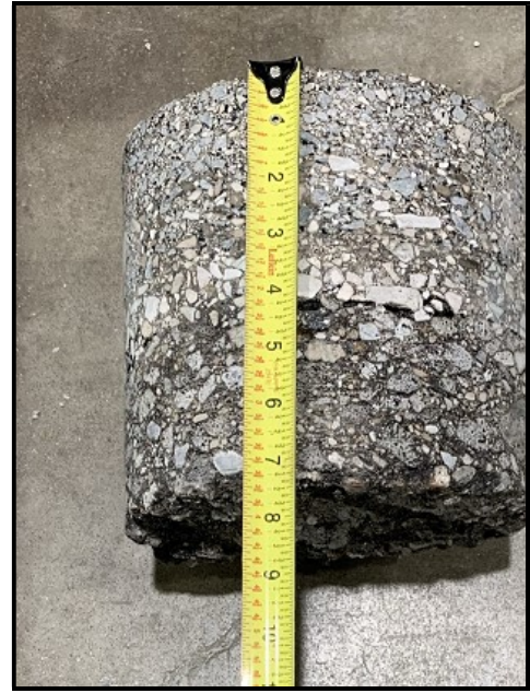
Coring No. B-013-0-20 Total Length: 7.250" Location: U.S. 422 W exit ramp STA 647+58 1' RT
