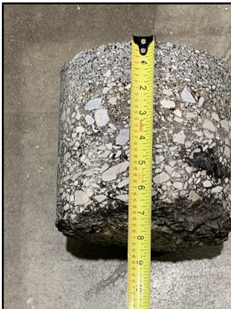
Coring No. B-014-0-20 Total Length: 7.500" Location: U.S. 422 W exit ramp STA 650+11 22' RT
