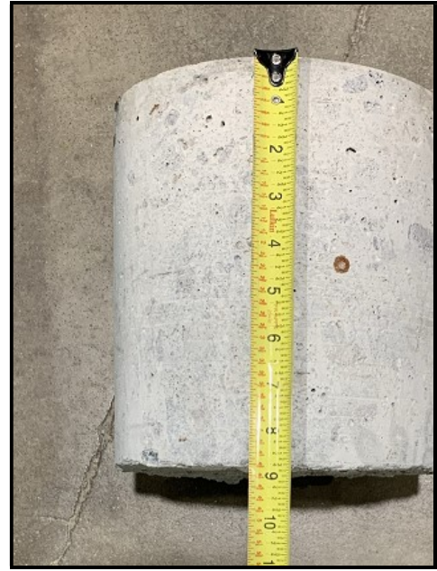
Coring No. B-006-0-20 Total Length: 9.000" Location: Harper Rd southbound curb lane STA 67+62 17' RT
