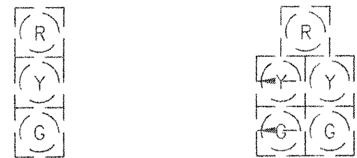
Signals A, B, D, E & F Signal C EXISTING SIGNAL HEAD ARRANGEMENT
