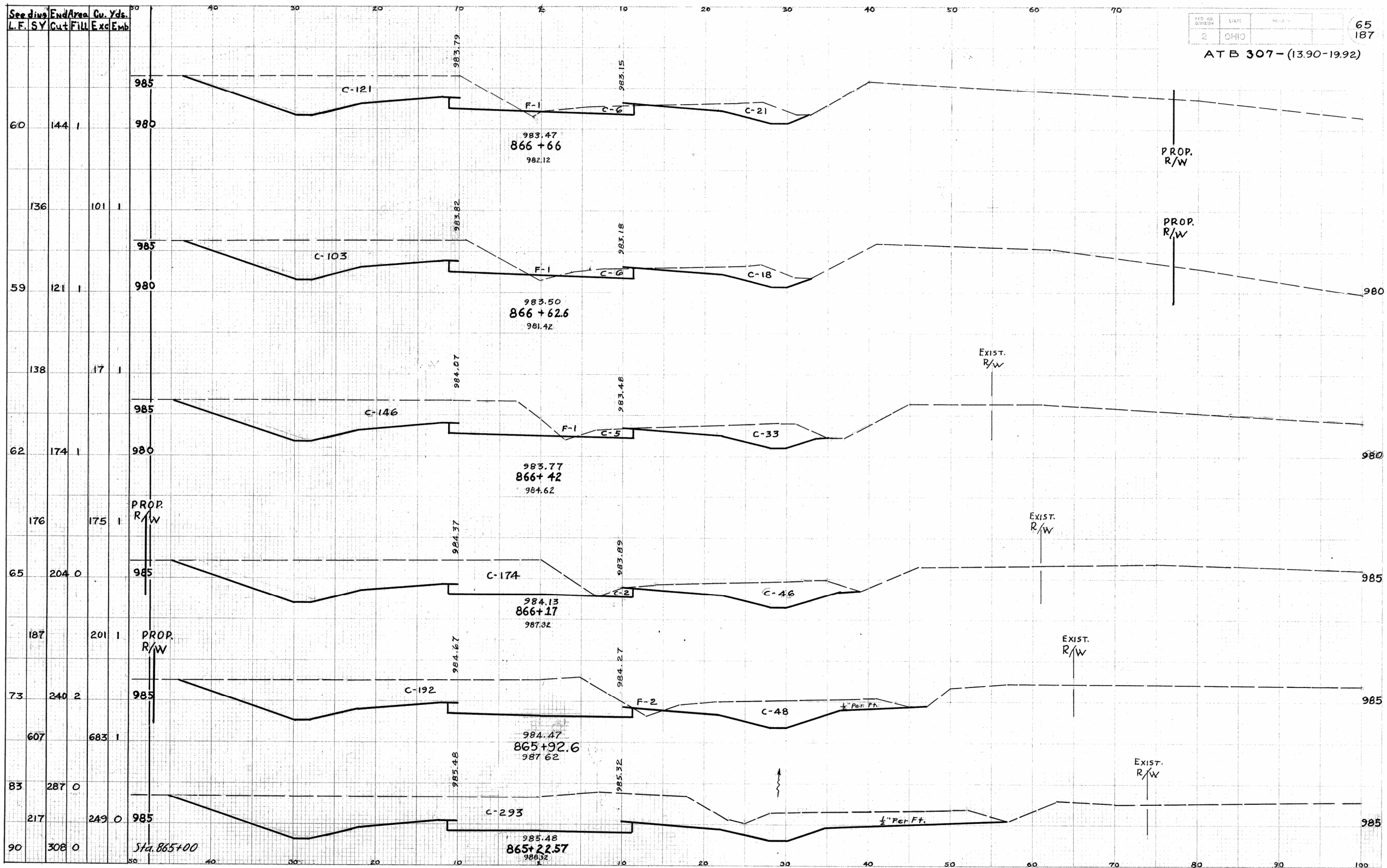
CROSS SECTIONS STA 865+22.57 TO STA 866+66
