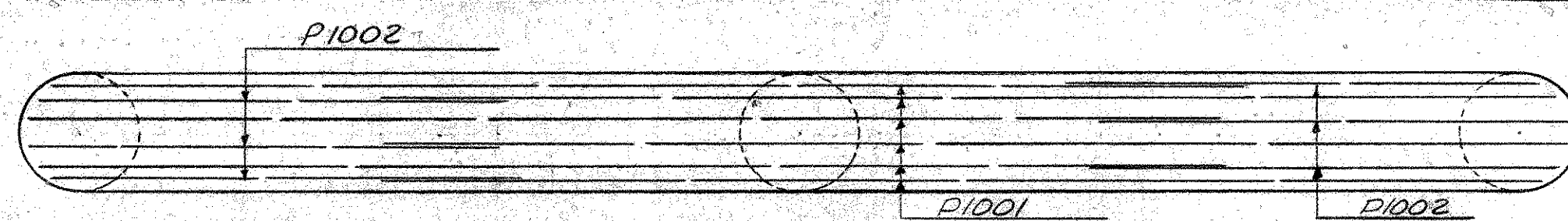
PLACEMENT DIAGRAM FOR P1001 AND P1002 IN TOP OF CAP
