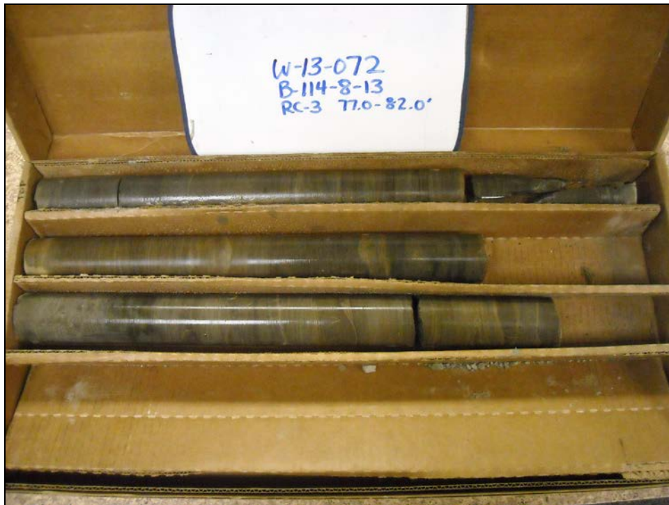
B-114-8-13 – RC-3 – Depth from 77.0 to 82.0 feet
