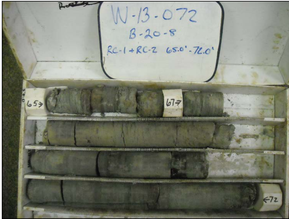
B-020-8-13 – RC-1 and RC-2 – Depth from 65.0 to 72.0 feet
