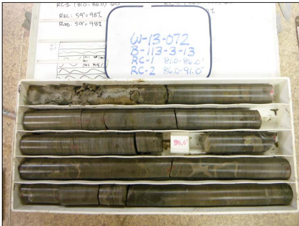
B-113-3-13 – RC-1 and RC-2 – Depth from 81.0 to 91.0 feet
