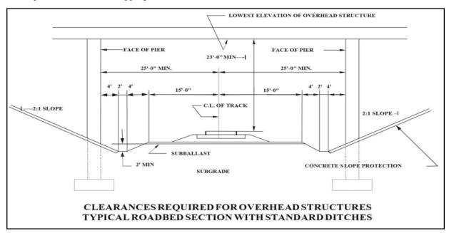
For multiple tracks, standard track centers are fifteen feet (15'-0") wide. An access road may be required to provide thirty-three feet (33'-0") minimum distance from the centerline of the track to the face of the pier.
