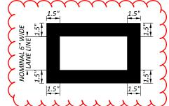
THE WHITE LANE LINE SHALL BE CENTERED ON THE BLACK MARKING SUCH THAT THERE WILL BE 1.5 INCH BLACK BORDER ON EITHER SIDE OF THE WHITE LANE LINE. THE WHITE LANE LINE SHALL BE CENTERED WITHIN THE BLACK PAINT AREA WITH BLACK ON BOTH THE LEADING AND TRAILING EDGES.
