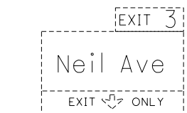
CANTILEVER MOUNTED SIGN
