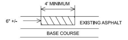
Existing deteriorated asphalt shall be removed to a maximum depth of 6 inches or as directed by the engineer and replace with Item 301, Asphalt Concrete Base, shall be compacted as per 401.15 and in approximately equal layers. The locations and size of the repairs shall be determined by the engineer.
