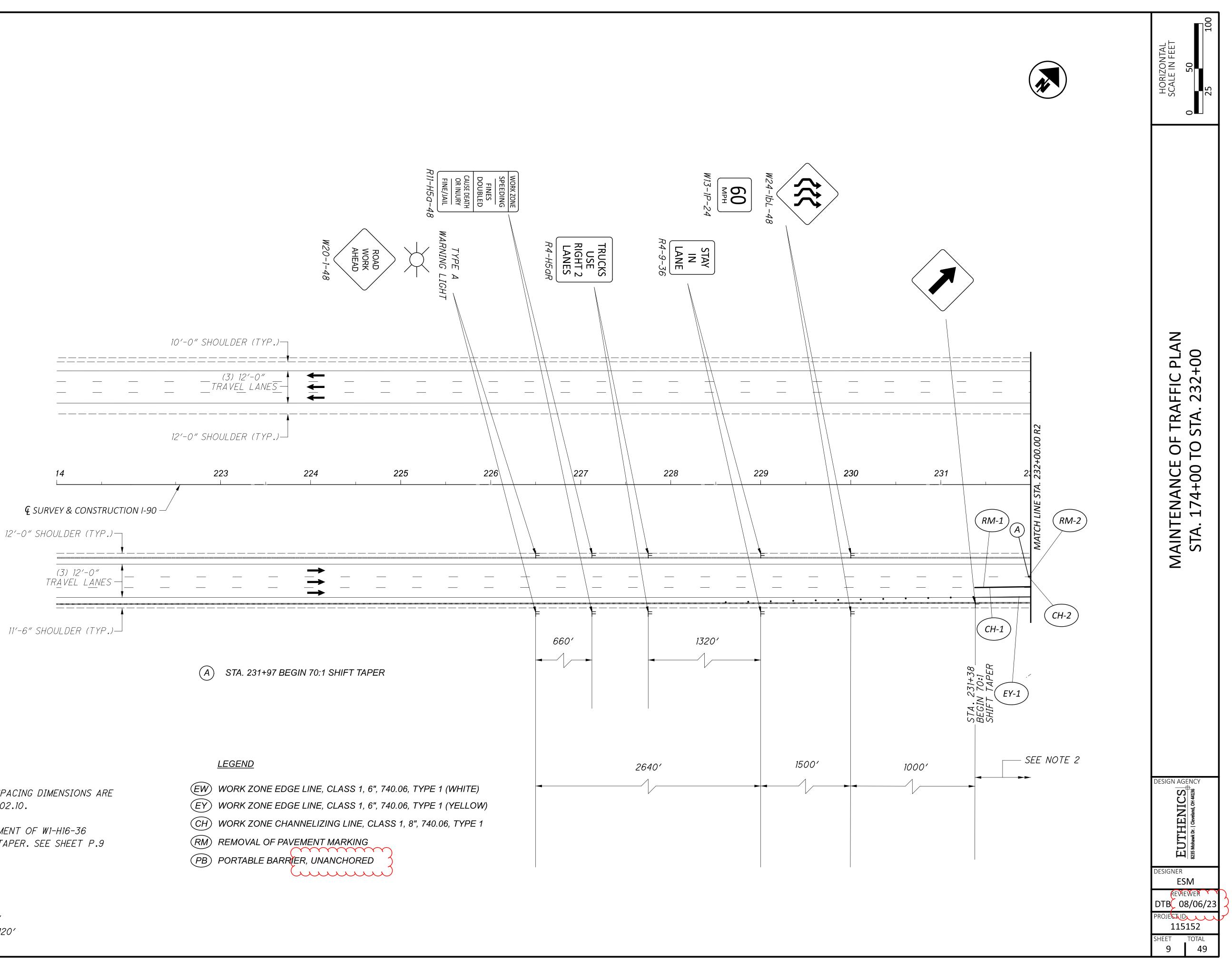
NOTES: 1. SIGN SPACING IS NOT TO SCALE. SPACING DIMENSIONS ARE SHOWN IN ACCORDANCE WITH SCD MT-102.10. 2. THE REQUIRED SPACING AND PLACEMENT OF WI-H16-36 SIGNS IS 100 FEET ALONG THE SHIFT TAPER. SEE SHEET P.9 FOR CONTINUATION. 3. PER SCD MT-102.10: -SHIFT TAPER RATE IS 70:1
