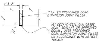
PAYMENT FOR THE ABOVE WORK SHALL BE MADE AT THE UNIT PRICE BID FOR ITEM 516 - 1" (or 2") PEJF, A.P.P., SO.FT., AND SHALL INCLUDE ALL LABOR, EOUIPMENT, AND INCIDENTALS REQUIRED TO COMPLETE THE WORK DESCRIBED.
