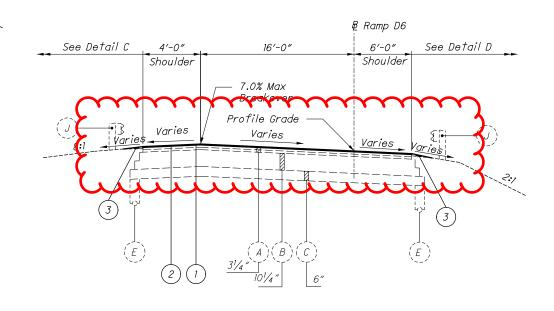
TYPICAL SECTION - Q SUPERELEVATED SECTION - Ramp D6
