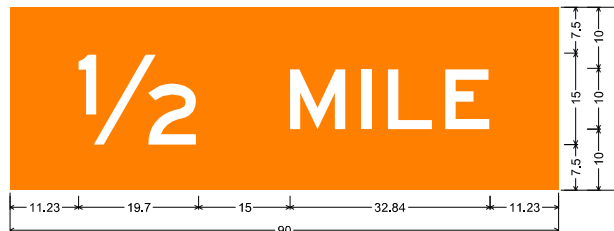
SN-129 LOCATED APPROX. AT SLM 5.87 No border, White on Orange; "1/2 MILE" Black, E;
