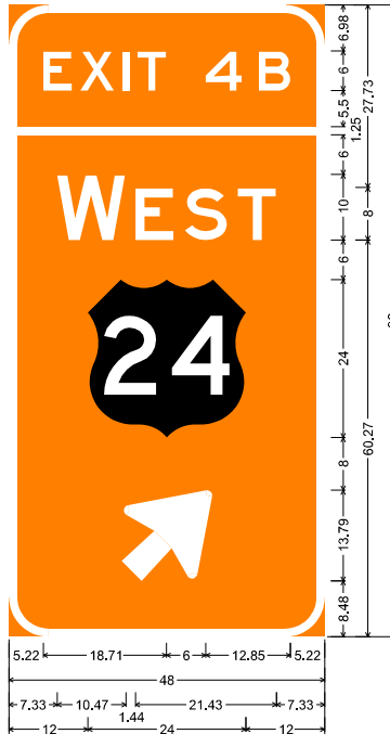
SN-103, SN-115, SN-125 6.00" Radius, 1.25" Border, Black on Orange; [EXIT 4B] E; [W] E; [EST] E; US 24 M1-4; Arrow B-4 - 17.00" 45";
