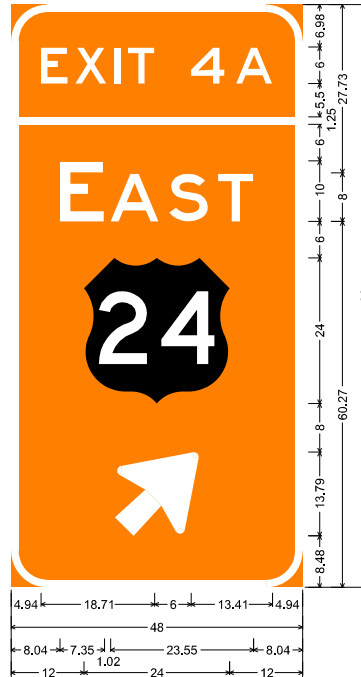
SN-102, SN-108, SN-113, SN-114, SN-124 6.00" Radius, 1.25" Border, Black on Orange; [EXIT 4A] E; [E]; [AST] E; US 24 M1-4; Arrow B-4 - 17.00" 45";
