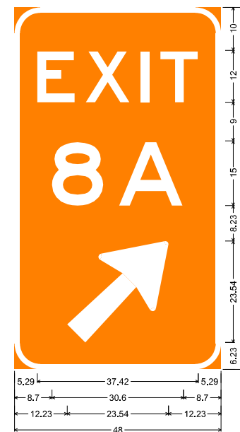
SN-121, SN-126 6.00" Radius, 1.25" Border, Black on Orange; "EXIT", E; "8A", E; Arrow A-2 - 30.00" 45";
