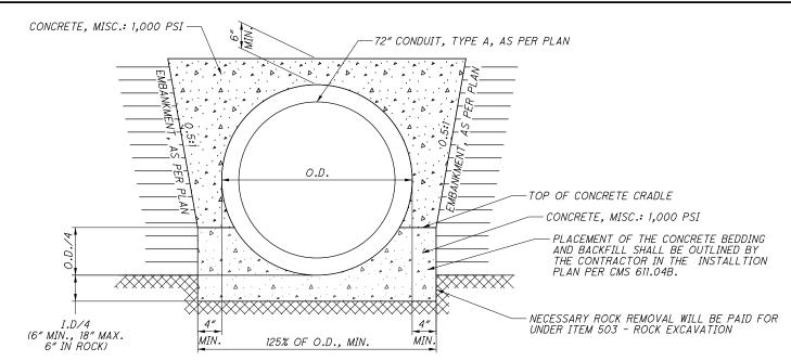
CONCRETE BACKFILL AND BEDDING DETAIL
