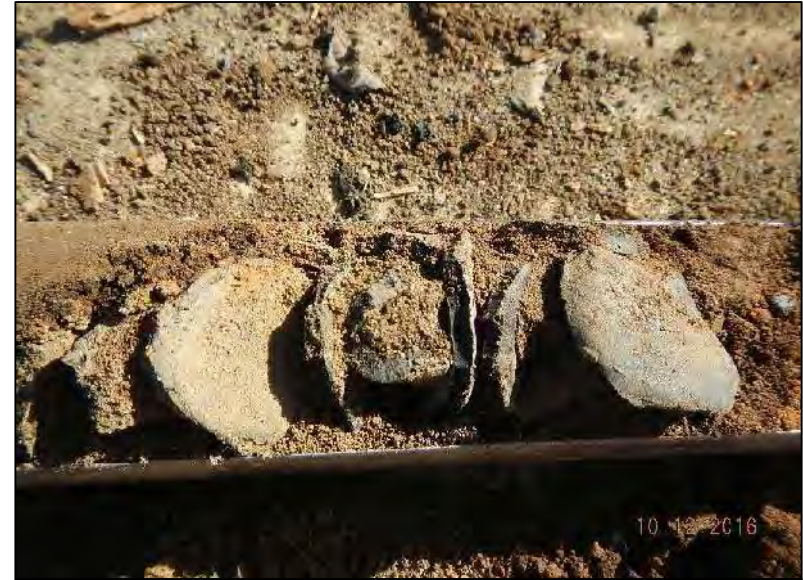
Photo 22 - Close up view of debris materials at EB-5 (crushed concrete, rubber, brick, carpet, built up roofing fragments).
