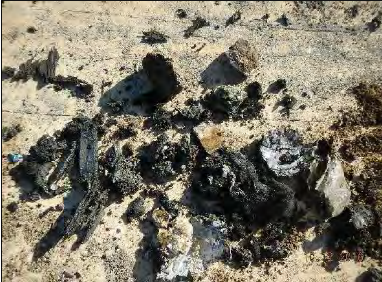
Photo 13 - Close up view of debris materials at EB-3 (wood, plastic, paper, fiberglass, and glass fragments).
