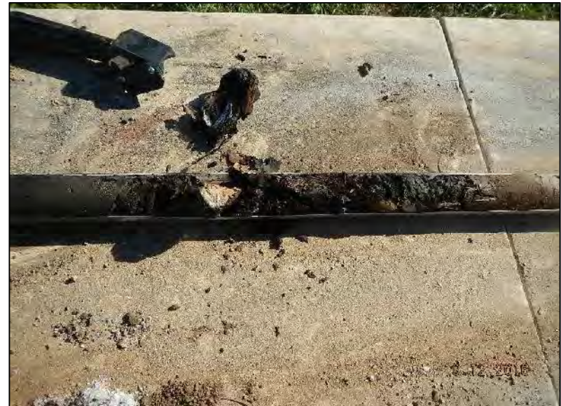
Photo 26 - View of soil profile at EB-6 (5-10' bgs) w/ plastic, wood, rubber, plastic fragments and organic matter. See soil boring logs for soil profile description.
