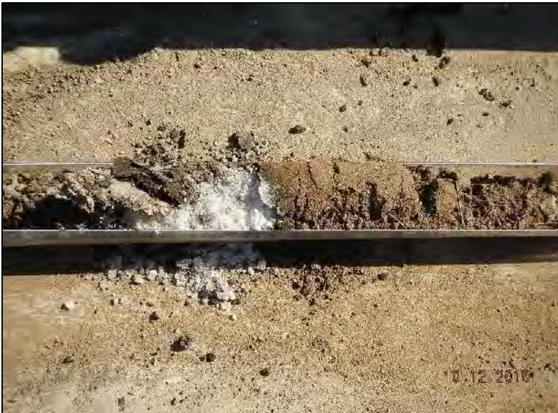
Photo 25 - View of soil profile at EB-6 (0-5' bgs) w/ plastic fragments and salt. See soil boring logs for soil profile description.
