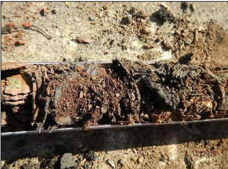
Photo 23 – Another close up view of debris materials at EB-5 (crushed concrete, rubber, brick, carpet, built up roofing fragments).
