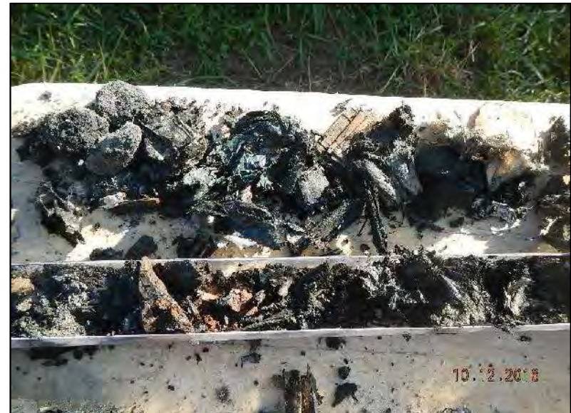
Photo 4 – Close up view of debris materials at EB-1 (plastic, rubber, wood, newspaper, landscaping waste).
