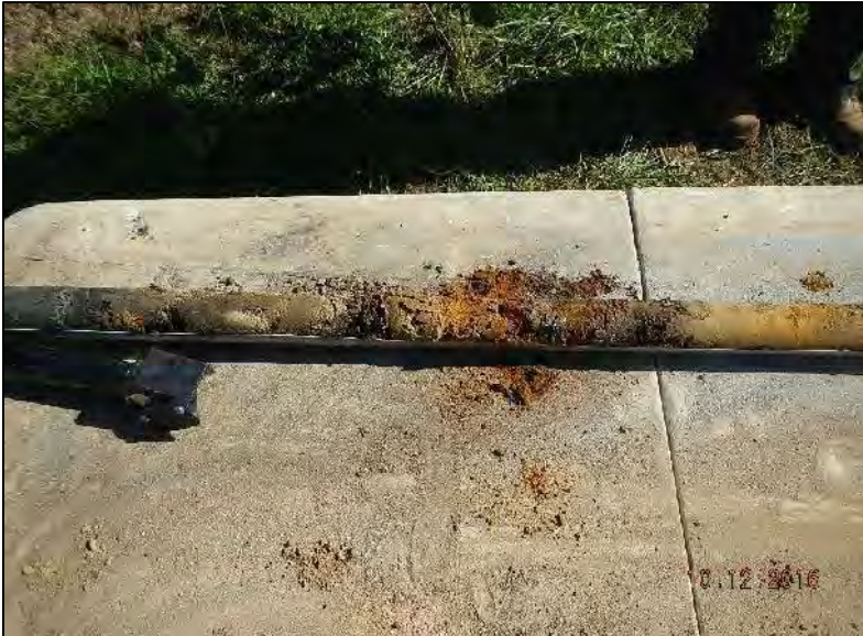
Photo 29 - View of soil profile at EB-7 (5-10' bgs) w/ brick and plastic fragments. See soil boring logs for soil profile description.
