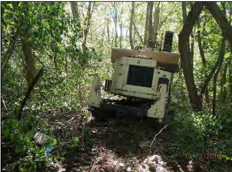
Photo 27 - View of Geoprobe drill rig set up at boring EB-7, facing east.
