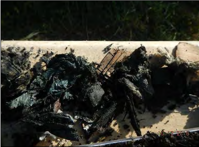
Photo 5 – Another close up view of debris materials at EB-1 (plastic, rubber, wood, newspaper, landscaping waste).
