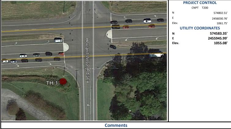
\* THE 4" STEEL GAS LINE IS MAKING A NOTICABLE UPWARD VERTICAL GRADE CHANGE IN A NORTHWESTERLY DIRECTION.
