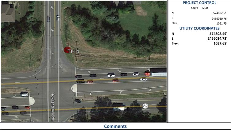
\* CREW COULD NOT DETERMINE IF THE ROUGH POURED CONCRETE IS A SHEATH OR DUCT. ELECTRONIC INFO PUTS THE 2" STEEL CONDUIT 1.4' DIRECTLY BENEATH THE CONCRETE.
