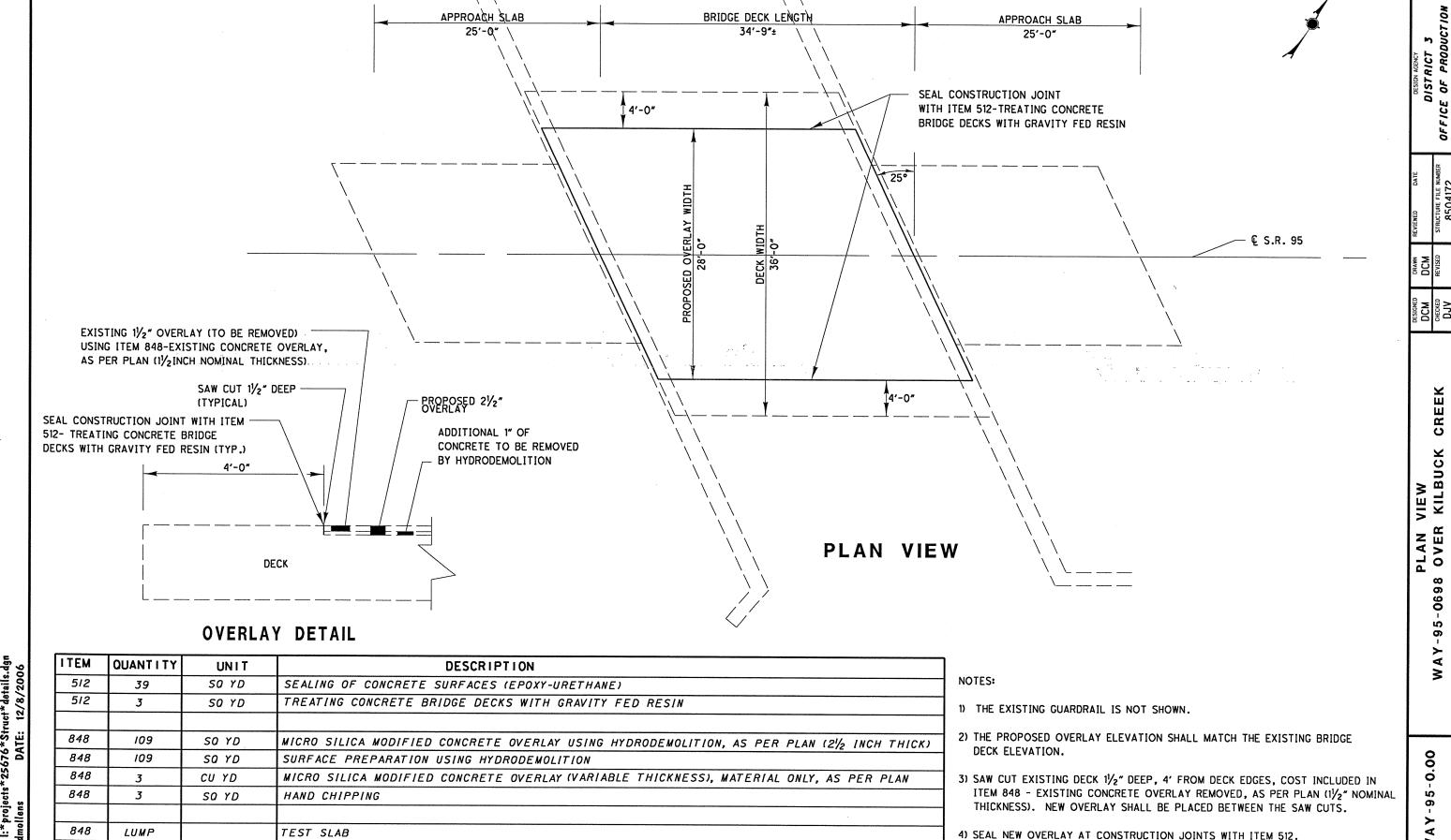
5) SEAL DECK EDGES AND ABUTMENT/WINGWALL (SEE SHEET 2/2 FOR DETAILS).
