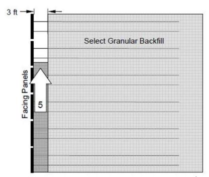
Figure 840.06-3 SGB Placement and Compaction Next to Facing Panels (Plan View)
