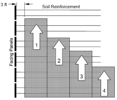
Figure 840.06-2 Procedure for SGB Placement and Compaction (Plan View)
