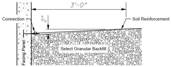
Figure 840.06-4 SGB at Connection
