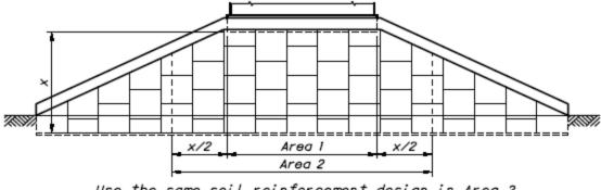
Use the same soil reinforcement design in Area 2 as that required under the footing (Area 1).
