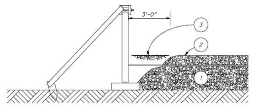
Figure 840.06-1 Backfilling for the First Row of Panels Only
