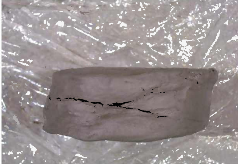
Post test picture, after pulling apart and putting back together. Shows development of an angular shear plane. Direct Simple Shear (DSS-2) test sample.
