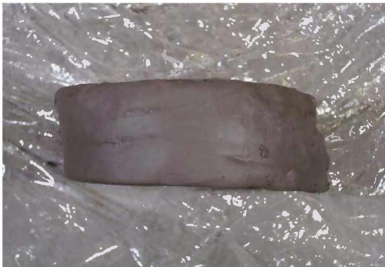
Post test showing failure lean to the left. Slight shear plane developing angling back. Direct Simple Shear (DSS-2) test specimen.
