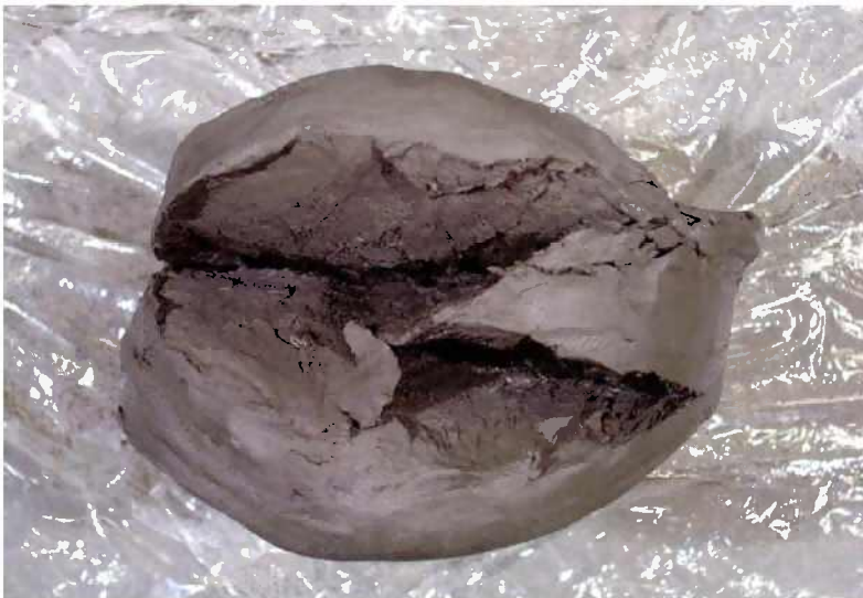
Same sample, pulled apart view of the internal structure along horizontal planes. The material appeared rough. There were no visible polished surfaces.
