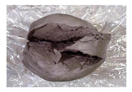
Same sample, pulled apart view of the internal structure along horizontal planes. The material appeared rough. There were no visable polished surfaces.
