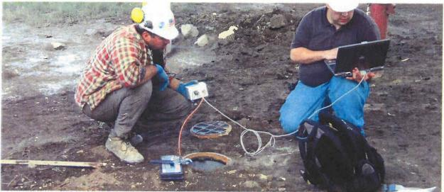
a) BBCM personnel performing an initial reading of a vibrating wire piezometer.
