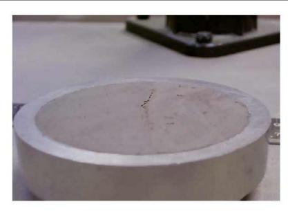
Sample in trimming ring showing an in-situ shear plane in the material as received. Residual Shear test (RS-2), angled view.
