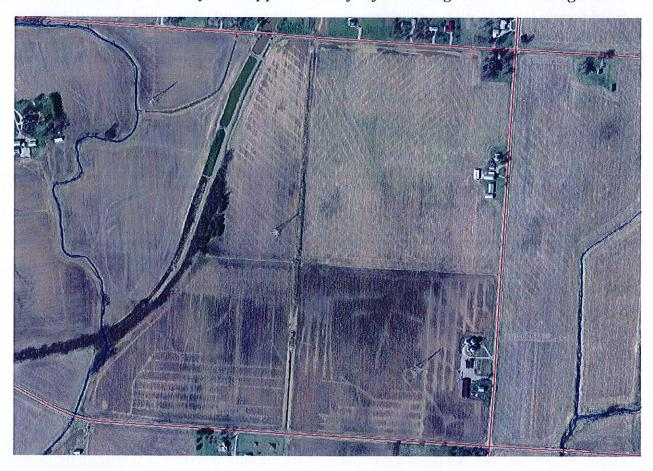
Above: Farm fields shown with systematic tile and random tile. The field with the systematic tile is much dryer than the one below it with random tile. Tile can be seen in aerials if soil conditions are right at the time of the flight. Plastic tiles tend to show up better than clay. Tiles are harder to see in grassed areas, like lawns on aerial photos.
