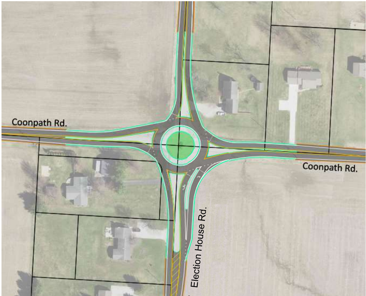
Figure 4 - Roundabout with right turn lane Schematic Plan View
