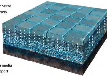
Stone or other storage media provides structural support and stormwater storage
